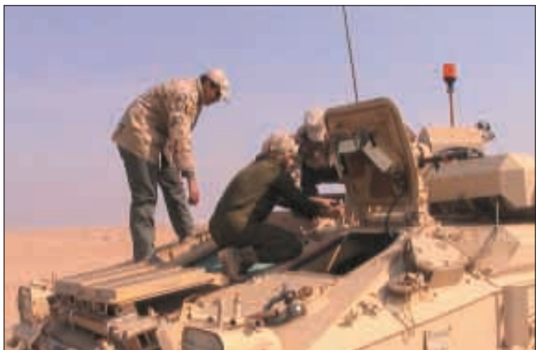
▲ Instructor Nigel Broadbent examines a Desert Warrior power pack with students on the vehicle mechanics course.
