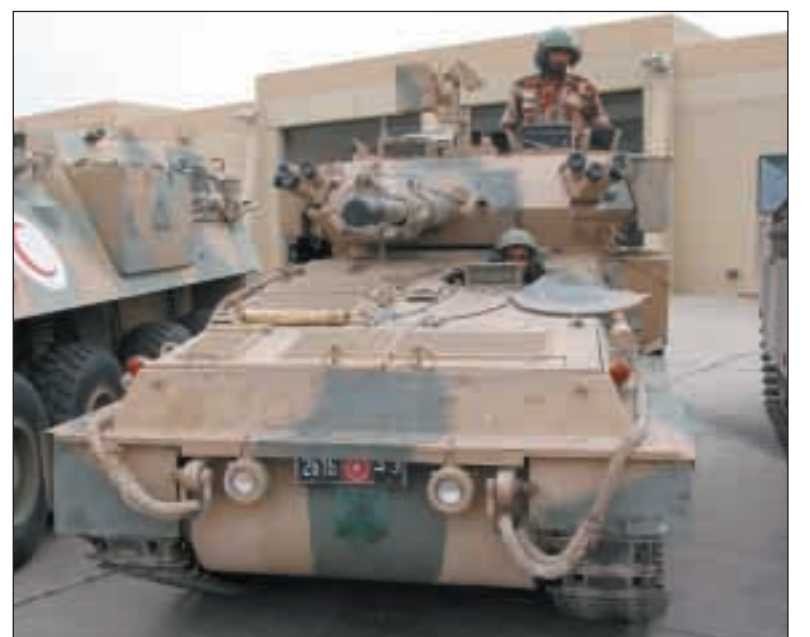
▲ Scorpion - one of a number of CVR(T)s being converted successfully to diesel.
