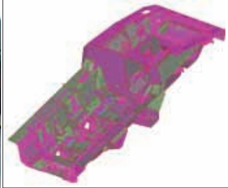
▲ Engineers at Telford have used finite element analysis in the design of the complex MRAV hull fabrication. The vehicle design has been optimised for maximum protection.
